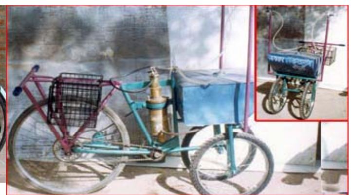
Bicycle based mobile spray pump Subhas Vasantrao Jagtap, Maharashtra
